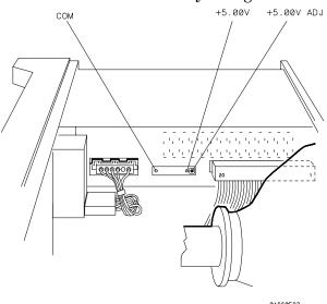
**6** Check for the voltages on the power supply cable using the values in the following table
